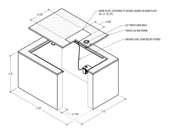
CONFORMANCE NOTE: THIS PRODUCT IS CONSTRUCTED AND TESTED TO CONFORM WITH WSDOT STANDARD SPEC. 9-29.2(1), STANDARD DUTY JUNCTION BOXES
