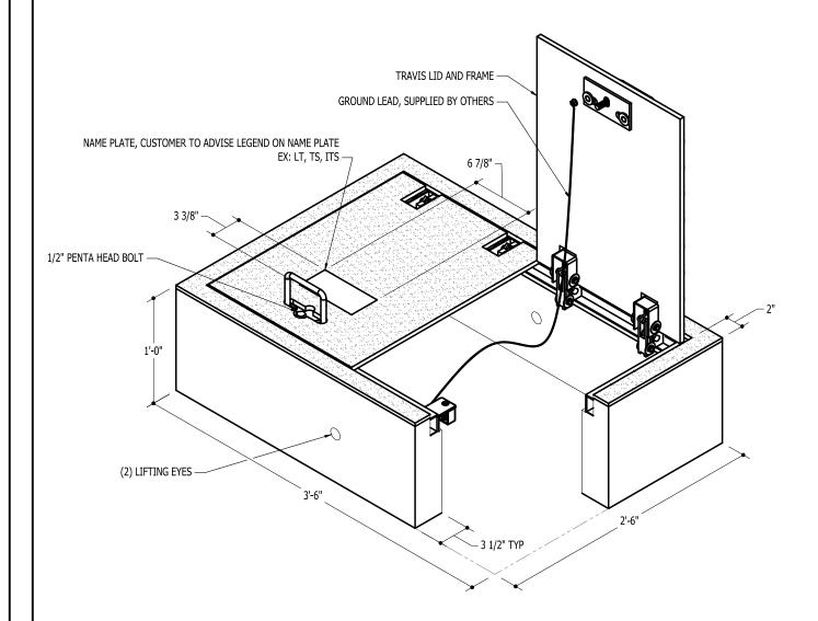
CONFORMANCE NOTE: THIS PRODUCT IS CONSTRUCTED AND TESTED TO CONFORM WITH WSDOT STANDARD SPEC. 9-29.2(1), STANDARD DUTY JUNCTION BOXES
