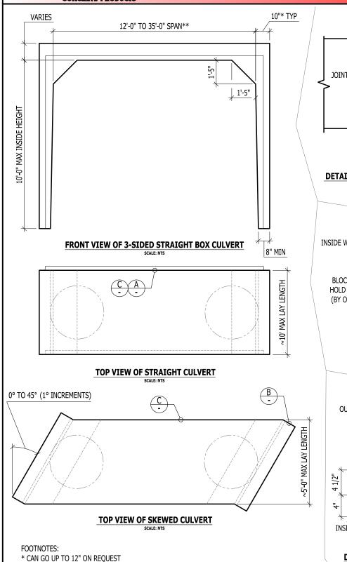
\*\* 1' INCREMENTS FOR STRAIGHT CULVERTS, SKEWED CULVERTS VARY BASED OFF OF SKEW
